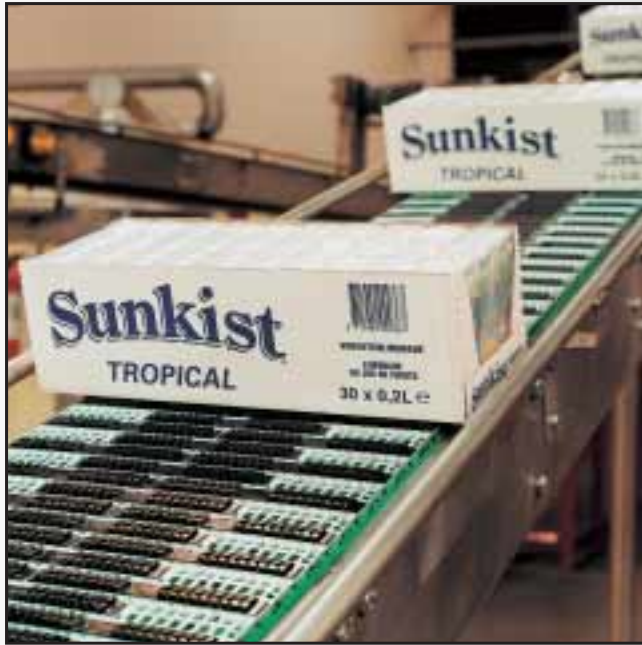
INCLINED TRAY CONVEYOR WITH PLASTIC SUPERGRIP BELT.
