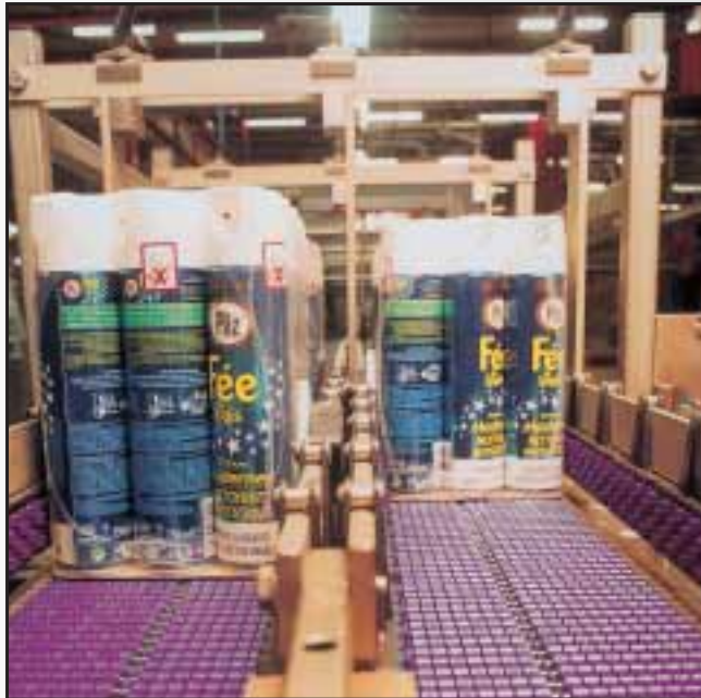
SMOOTH MULTI-PACK CONVEYOR WITH PLASTIC LBP CHAIN.
