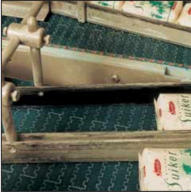
HEAVY DUTY SUGAR SACKS CONVEYOR WITH PLASTIC 1005-SERIES BELT.
