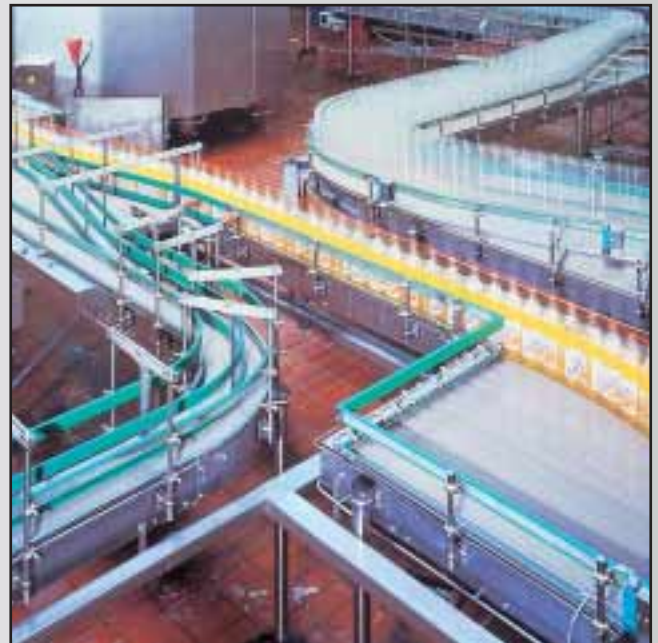
PET BOTTLES ON SOFTLINE BEVELLED SINGLE HINGE CHAIN.
