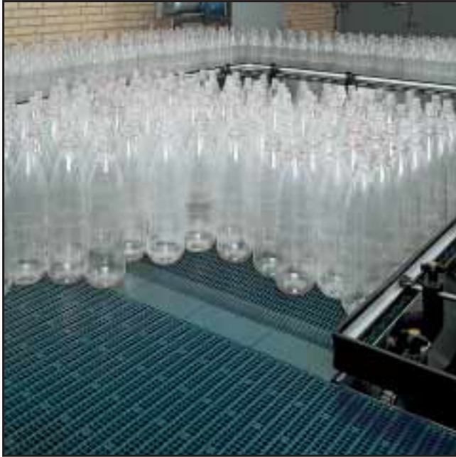
SMOOTH BOTTLE TRANSFER WITH PLASTIC CLICK-COMB FINGERPLATES.
