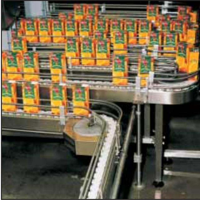
TYPICAL CARTON CONVEYOR WITH PLASTIC MULTIFLEX CHAIN.
