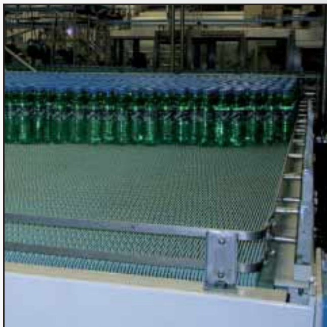
BOTTLE CONVEYOR WITH PLASTIC 2000-SERIES BELT.
