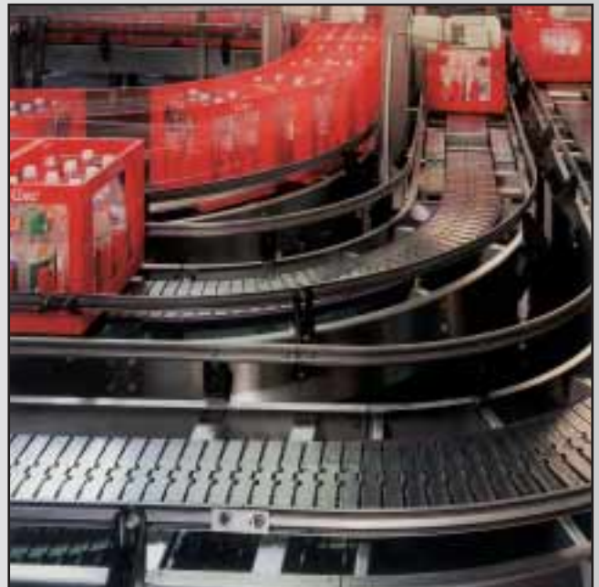
CASES ON WEAR-RESISTANT 60-SERIES MAGNETFLEX® CHAIN.
