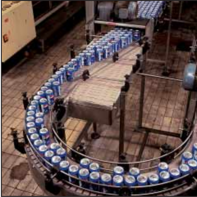
HIGH-SPEED, HIGH-CAPACITY CAN CONVEYOR WITH PLASTIC MAGNETFLEX® CHAIN.
