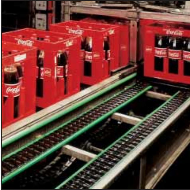
HEAVY DUTY CRATE CONVEYOR WITH STAINLESS STEEL CHAIN WITH RUBBER TOP.
