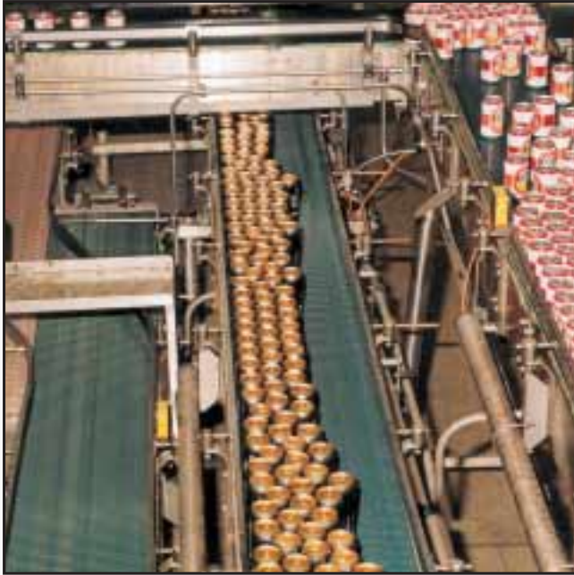
SMOOTH CAN CONVEYORS WITH 500-SERIES PLASTIC BELT.
