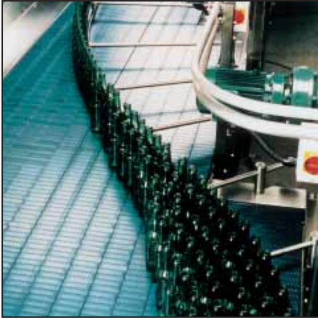
EMPTY GLASS BOTTLE CONVEYOR ON INLINER WITH 1000-SERIES PLASTIC BELT.
