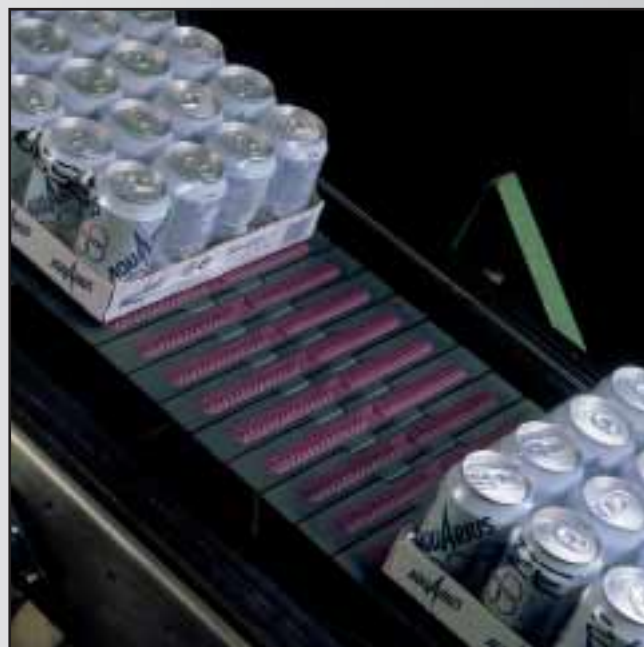
TRAYS WITH CANS ON HIGH FRICTION 12" SUPERGRIP CHAIN.
