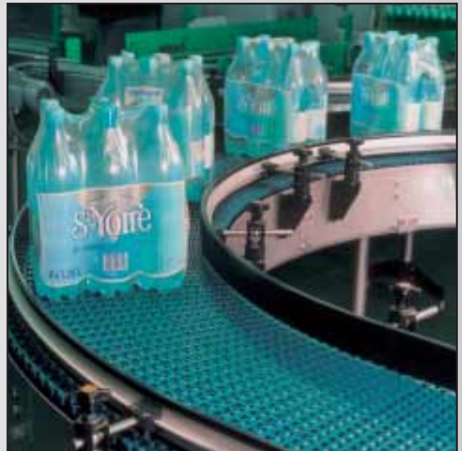
SHRINK-WRAPPED BOTTLES ON 1255-SERIES FLEXBELT.
