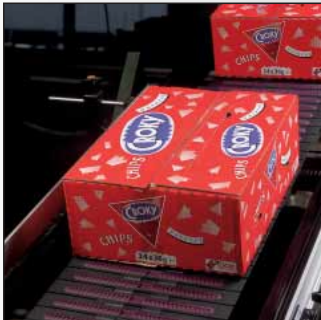
INCLINED BOX CONVEYOR WITH PLASTIC SUPERGRIP CHAIN.
