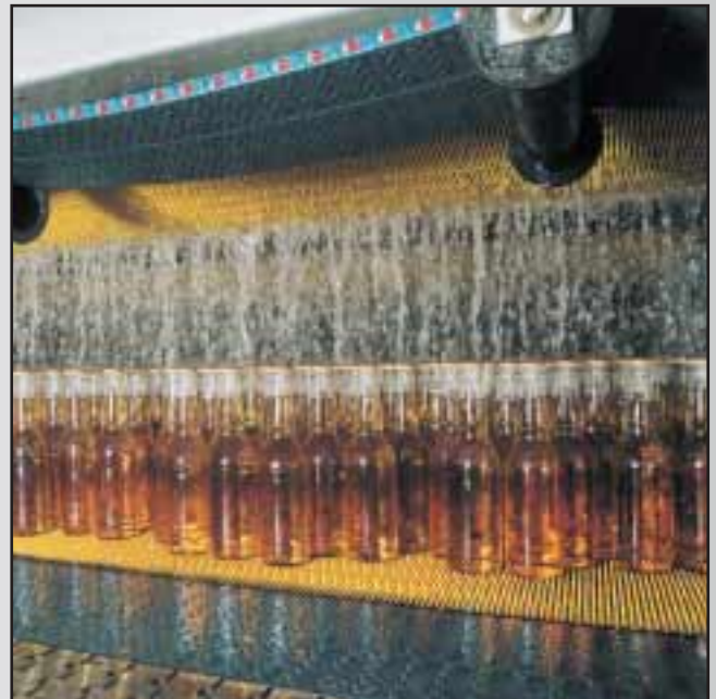
SELF-CLEARING DTS-C SYSTEM IN A PASTEURIZER INFEED.
