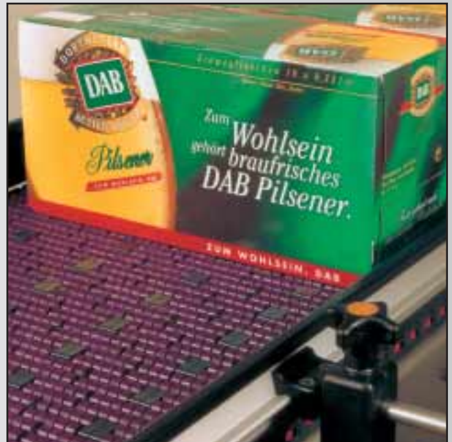
LARGE PACKS HANDLED WITH CARE ON QUIET 1005 LBP BELT.
