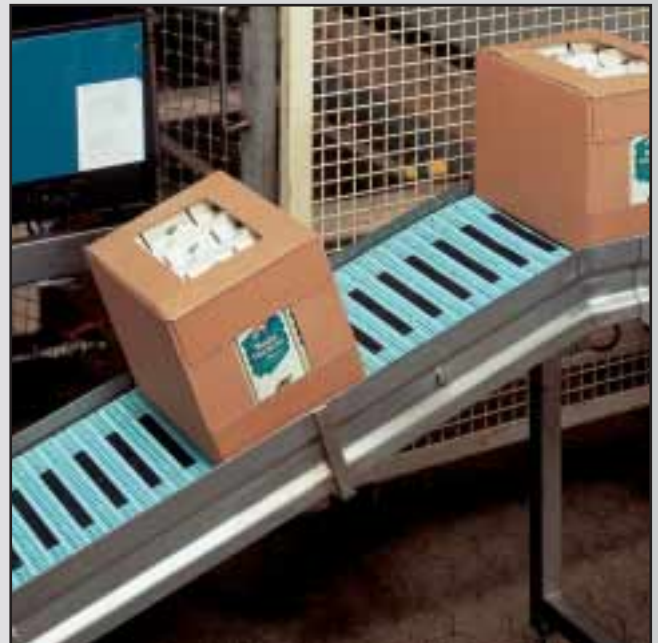
BOXES WITH CARTONS ON PARTIALLY RUBBER COVERED SUPERGRIP BELT.
