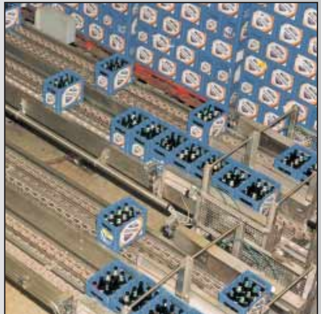
CRATES WITH RETURNED BOTTLES ON OPEN, HYGIENIC CC 1400 CHAIN.
