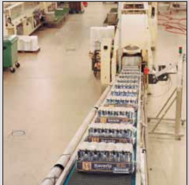
HEAVY TRAYS ON SIDE-INDENT 1005 SUPERGRIP BELT.
