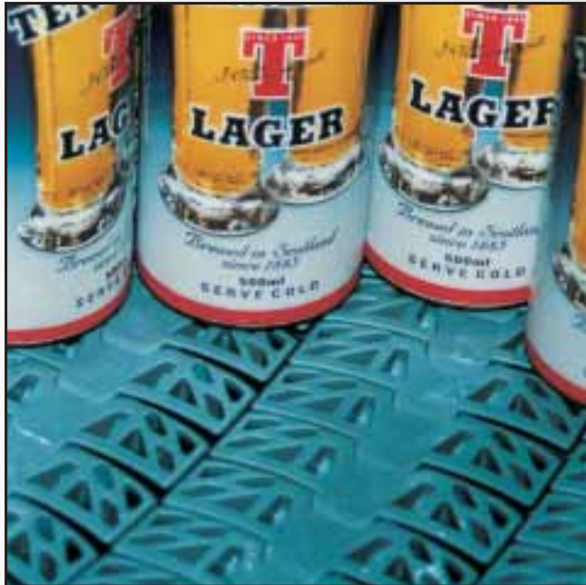
SIDEFLEXING CAN CONVEYOR WITH PLASTIC MAGNETFLEX® 1050 CHAINBELT.
