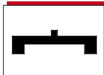
Part. 263 - Page 10 Chain guide profile. Multiple strands K82,5 / pitch 88
