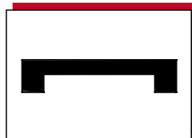
Part. 387 - Page 11 Chain guide profile. Multiple strands K87 / pitch 88
