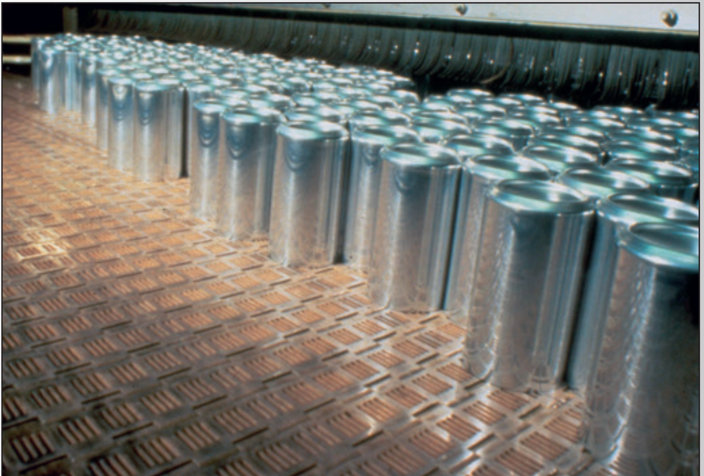
CAN CONVEYOR WITH 5706 BELT
