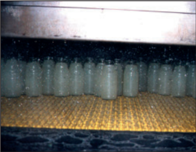
BOTTLE PASTEURIZER INFEED WITH 2500 BELT
