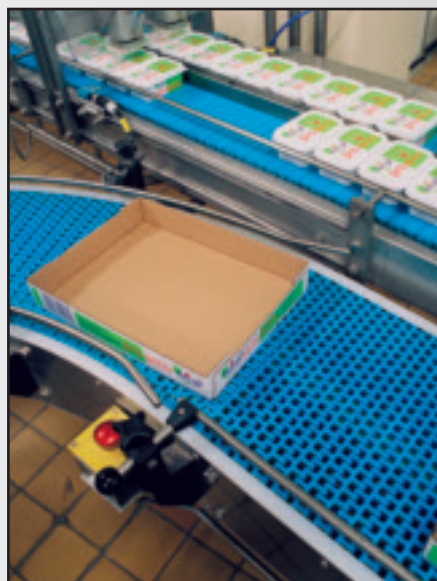
BUTTER TUBS PROCESSING ON 1255 BELT
