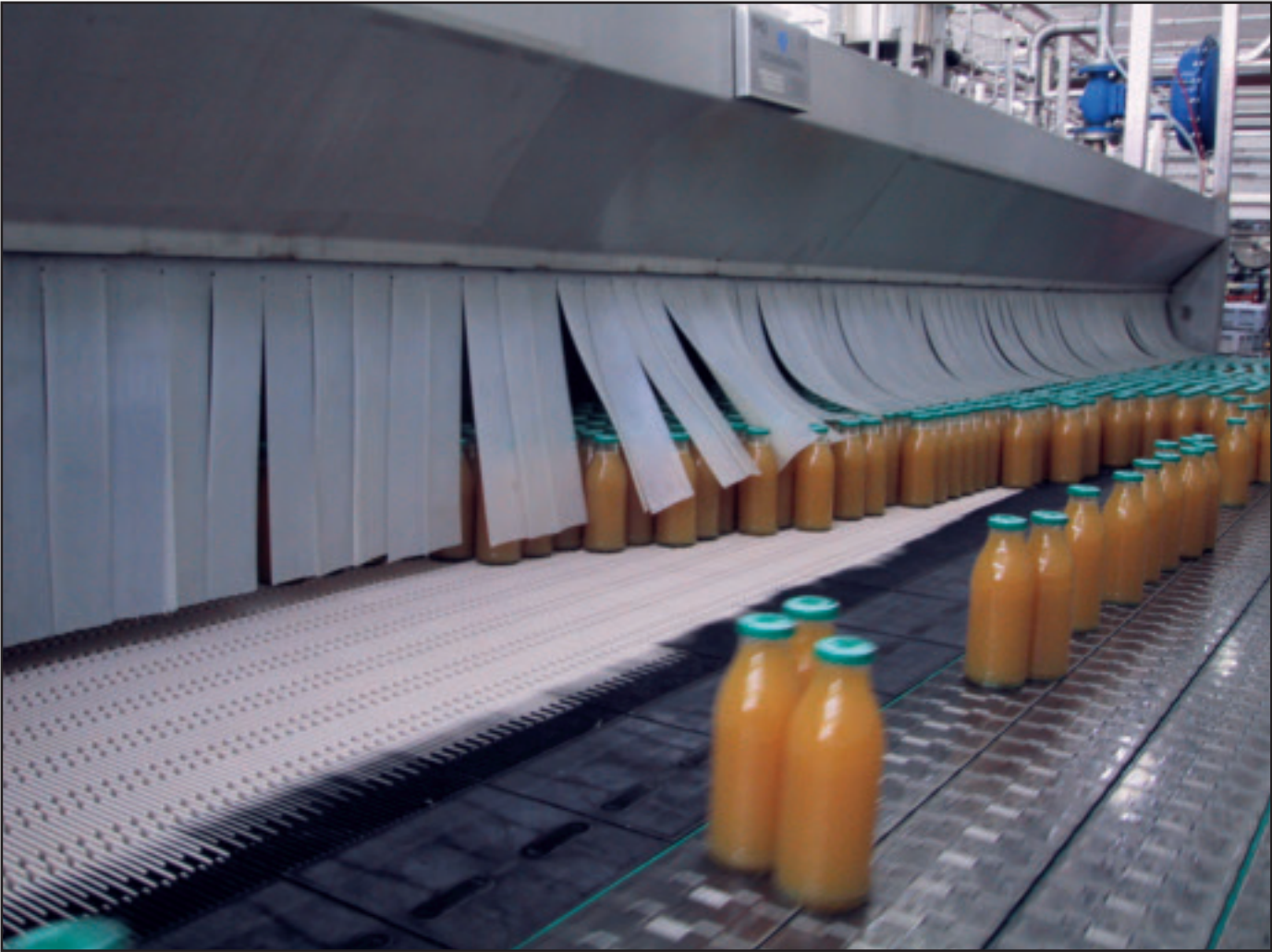
CAN PASTEURIZER WITH 4809 BELT
