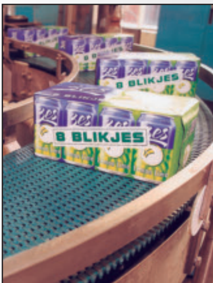
SHRINKWRAPPED PACK CONVEYOR WITH 505 BELT
